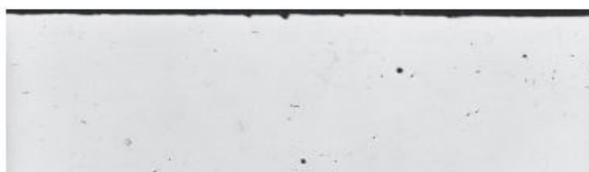
HAYNES® 214® alloy Average Metal Affected = 0.5 mils (13 µm)
