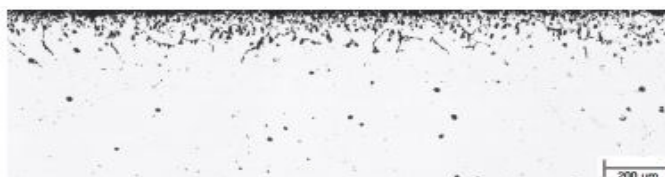
RA330® alloy Average Metal Affected =8.7 mils (221 µm)
