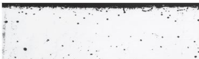
Alloy 600 Average Metal Affected =4.8 mils (122µm)
