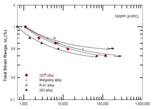
1500°F (816°C), Fully Reversed, R = -1, Waveform = Triangle, Frequency = 0.33Hz, Material: 0.125"(3.2 mm) Sheet\*
