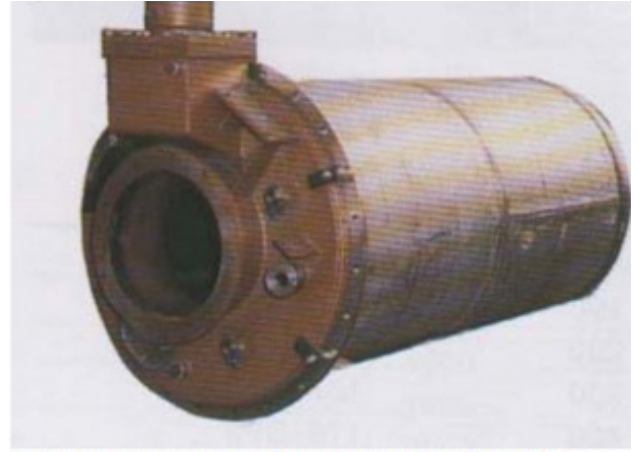
56 alloy vacuum carburizing furnace retort.
