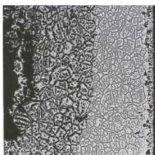
INCONEL alloy 601 Average Metal Affected = > 22 Mils (560 µm)/Side
