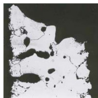
alloy 600 Average Metal Affected = > 22 Mils (560 µm)/Side
